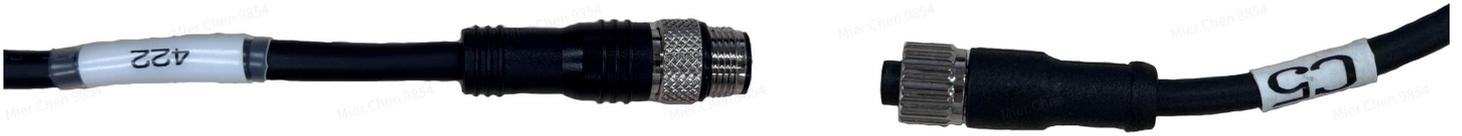
2. Connect the 4-pin connector labeled "C3" on the signal conversion harness ⑤ to the 4-pin connector labeled "CAN 250K" on the VCU wiring harness ⑥.
